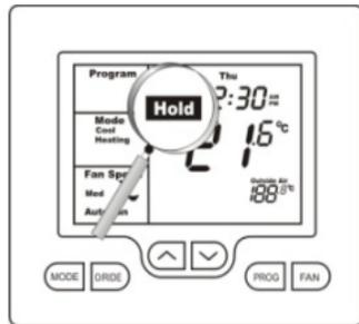
If desired, while the program is held the current set temperature can be adjusted simply by pressing and holding the up (▲) or down (▼) buttons for 3 seconds. The Chameleon thermostat display will change to show the word **“SET”**, and the active set point for the current mode. (Heating or Cooling) as you hold the up (▲) or down (▼) buttons the current set point will change.
