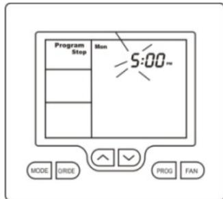
Tap the **“PROG”** button again, now the minute’s digits flashes. Using the up (▲) or down (▼) buttons set the minute to the time you wish the building air conditioning system to **“STOP”** for the currently selected day. The LCD will now show the word **“COPY”**.
