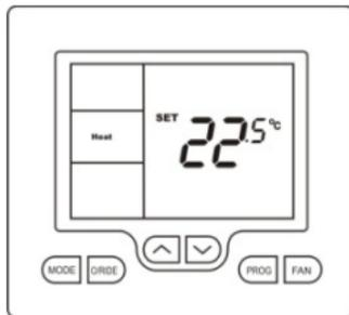
If Auto mode is selected, after adjusting the Heat set point wait without touching a button for 3 seconds for the Chameleon thermostat display to change to show “Cool” and “SET” and your current cooling set temperature. If desired change this value with the up (▲) or down (▼) buttons. Again wait for three seconds to exit the temporary overridden programmed mode.
