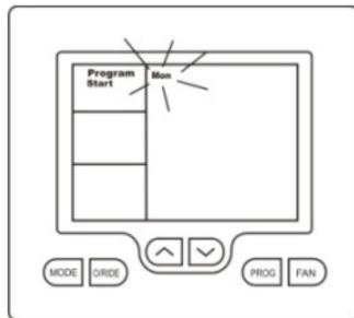
Tap the **“PROG”** button to advance to the next step, The LCD will show the word **“START”** with the hour’s digit flashes. Using the up (▲) or down (▼) buttons adjust the hours value to the time you wish the building Air Conditioning system to start.
