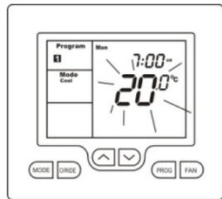
Tap the **“PROG”** button again, now the word **“HEAT”** (if enabled by the installer) and a temperature value is shown in the LCD, using the up (▲) or down (▼) buttons set the desired heating temperature to be maintained for the number **“1”** event.
