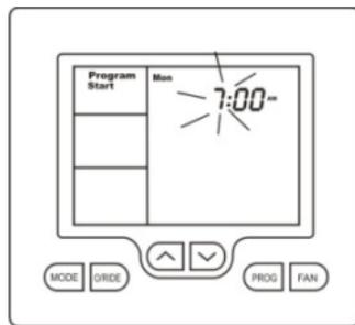
Tap the **“PROG”** button to advance to the next step, The LCD will show the word **“STOP”** with the hour’s digit flashes. Using the up (▲) or down (▼) buttons adjust the hours to the time you wish the building air conditioning system to **“STOP”** for the currently selected day.
