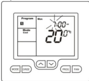
LCD will show the digit **“1”** with the hour's digit flashing. Using the up (▲) or down (▼) buttons adjust the hours to the time you wish the number **“1”** event to commence for the currently selected day.
