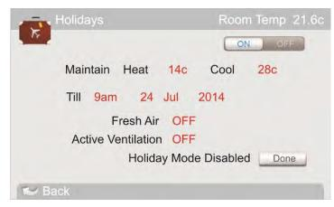
return. Then simply select ON. The Inspire Touch will open all zones and control your heating and cooling system to maintain your desired temperatures as measured at wall controller 1.
