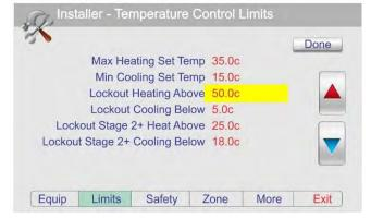
show it has been selected Lockout Heating Above in the above example). Use the up/down button to scroll through the options or values available for that option selected. Press "DONE" to save the change.
