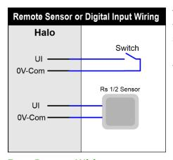
The SMT-850 HALO™ has four universal inputs that have a library of functions. These inputs will accept a digital input (switch input), a standard Smart Temp temperature sensor or a 0-10V input.
