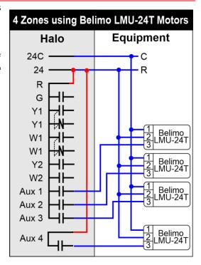
In this example, the SMT-850 HALO $^{\text{TM}}$  is switching 4 dampers. The SMT-850 HALO $^{\text{TM}}$  can control from 1 to 4 zones.
