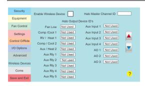
When wiring control relays, remote temperature sensors, or 0-10V analogue outputs for valves, dampers, or other Halo IO devices is difficult, wireless alternatives are available. This wireless version features an optional LoRa (Long Range) radio that pairs directly with the SMT-850 Halo and remoted devices via radio frequency signals (up to 1 km outdoors). These wireless devices operate in parallel with the SMT-850
