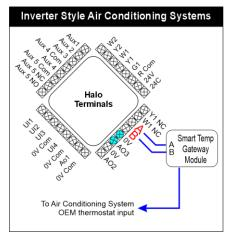
The SMT-850 HALO™ can control many inverter AC systems by using a protocol adapter to convert standard ModBus RTU communications from the SMT-850 HALO™ into the language required by the various brands of Air Conditioning systems. There are several brands of protocol adapters supported by the SMT-850 HALO™ however they are a wired to the SMT-850 HALO™ in the same manner.
