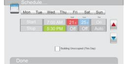
You are NOT permitted to adjust the "Stop" schedule heating and cooling temperature and fan modes. These are protected in the installer menu and can only be set in the Installer Options Window. The current values that the installer has set are displayed. See page 37 for information on setting the "Stop" event temperatures.
