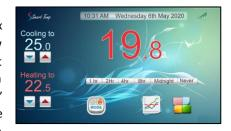
period such as 2 hours, the SMT-850 HALO™ will automatically set the thermostat mode to OFF in two hours. A reminder will be shown on the Window indicating the time of day the SMT-850 HALO™ will turn off.
