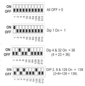
Hint. When setting codes on the DIP switch, start with the Dip that has the biggest number that is equal to or is smaller than the largest DIP switch value. Then the next largest number that will take as much of the remainder as possible and continue until you reach the code you desire.
