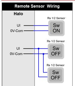
The SMT-850 HALO™ can measure space temperatures in multiple locations to improve the comfort level in the home or office. These sensors can be used individually or grouped together if an average temperature over a larger area is required.
