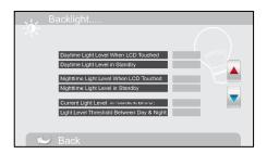
Note - If you have the Photo setting enabled the backlight level set in this menu will affect how the photo is displayed.
