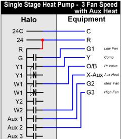
Auxiliary Heat uses the W2 as the "next" stage of heating in Aux heat mode.
