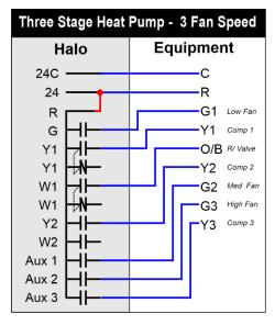
You will need enter the installer options menu, under the IO options tab and select Auxiliary relay 3 and assign its function as compressor 3
