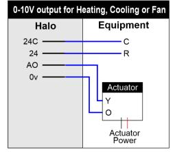
This drawing shows the wiring for a typical 0-10V actuator that may be used for a water valve or for damper control for example.
