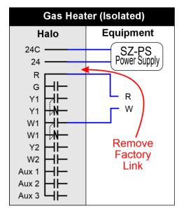
If your gas heater does NOT have a 24V C terminal or it requires a purely volt free input, you will require 4 wires between the SMT-850 HALO™ and the gas heater and a separate 24V AC/DC power supply such as the Smart Temp SZ-PS
