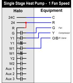
Single Stage Heat Pump is a quite common use of the Inspire. Note – SW4 sets revering valve logic.
