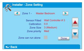
Zone control in the Inspire Touch is simple to use and understand, offering 3 zone control modes. A basic mode (Non Adjustable), where all zones are maintained to the same temperature; A simple mode, (open / close of zones only permitted) where all zones are maintained to the same temperature however you can select zones as open (on) or closed (off) and a more advanced mode, where all zones are completely individual - each zone with the ability to have individual schedules and temperatures.
