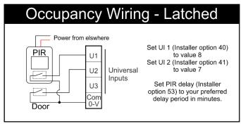
occupied, such as in a hotel room while the guest sleeps. During these periods of inactivity in the space you do not wish the Heating, Cooling or Air Conditioning to shut down.
