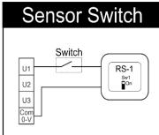
A typical maximum of 40 meters is permitted for sensor runs with 0.3mm or larger shielded cable should be used.
