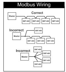
single hub. Each SMT-400 on the hub must have a unique network address (factory default is 7). These settings are adjustable from the advanced installer menu. See installer options 54, 55 & 56 on page 23 for more detail on setting the communications address.
