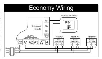
When Economy Cycle is <u>not</u> being used the Fresh Air damper output will be 0v. The Return Air damper will be at 10v. (The sum of both outputs always = 10V)
